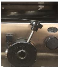
7. Bring the knife close to the specimen by pressing the rapid advance buttons outside the chamber. Use the advance handle (wheel on right hand side of cryostat) to raise and lower the specimen as you are positioning the knife close to it.
