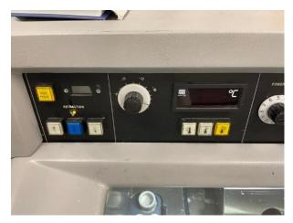
If the specimen head does not move, verify that the power to the motor control is on (green light in the picture below)
