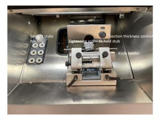
If the chuck is very close to the knife holder, retract it by pressing the rapid retract button to the left, outside the chamber.
